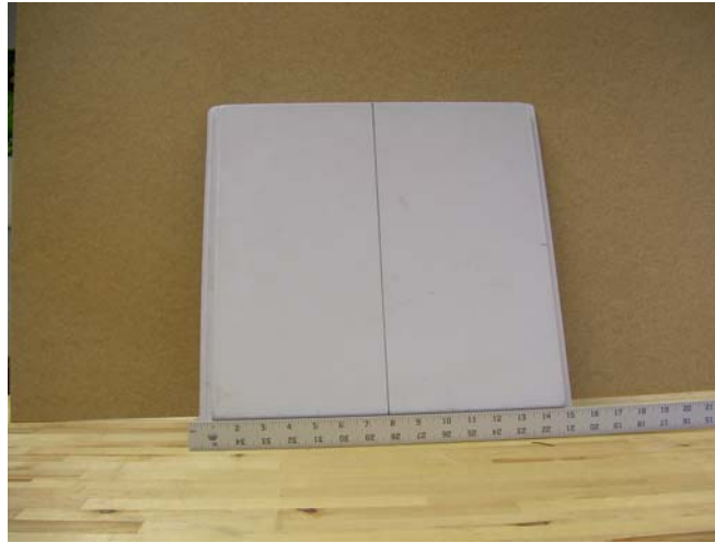
Figure 3.5: 19 dBi Yagi patch antenna used for receiving wireless energy transmissions from the helicopter.
