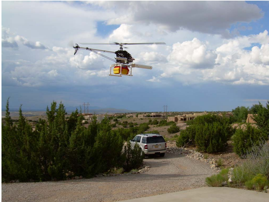
Figure 4.15: Initial test of helicopter load bearing capability.
