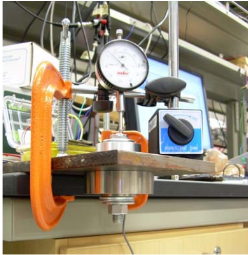
Figure 2.13: Bolted joint preload sensor test setup
