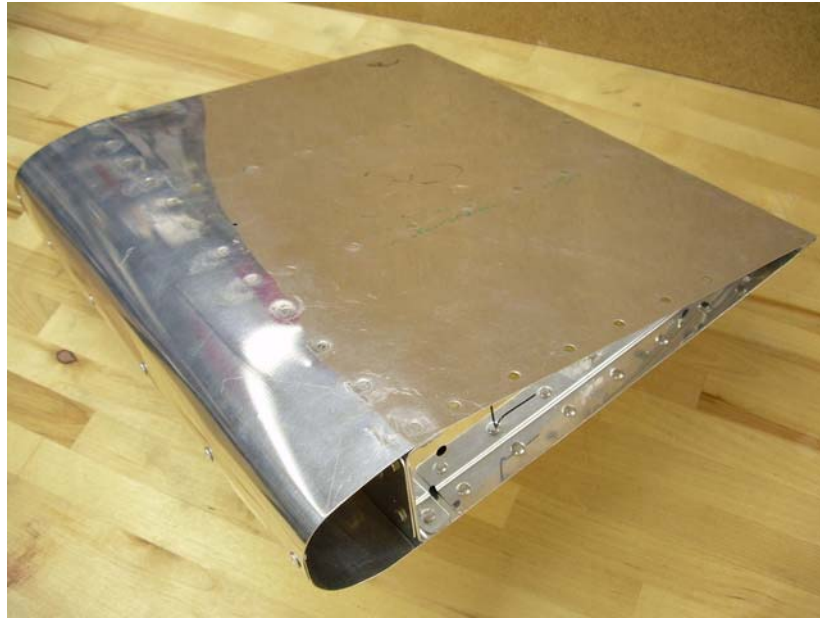
Figure 4.11: Sheetmetal construction typical of experimental homebuilt aircraft.
