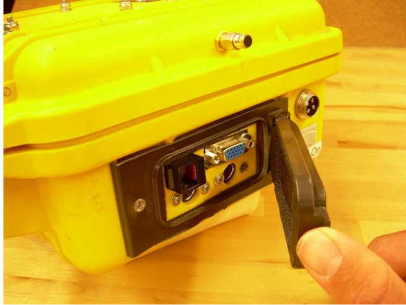
Figure 4.10: Spring Loaded Cover to Protect Connectors From Dust and Debris
