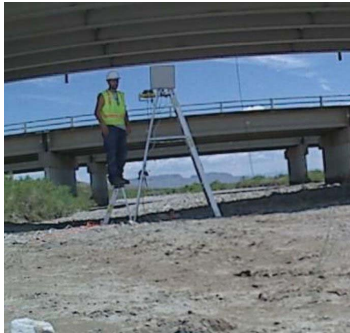
Figure 3.25: THINNER sensor node moved closer to ground level.
