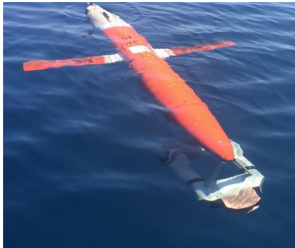
Figure. 1.1. Zooglider on deployment off of Mission Bay, CA (Photo: B.M. Whitmore).
