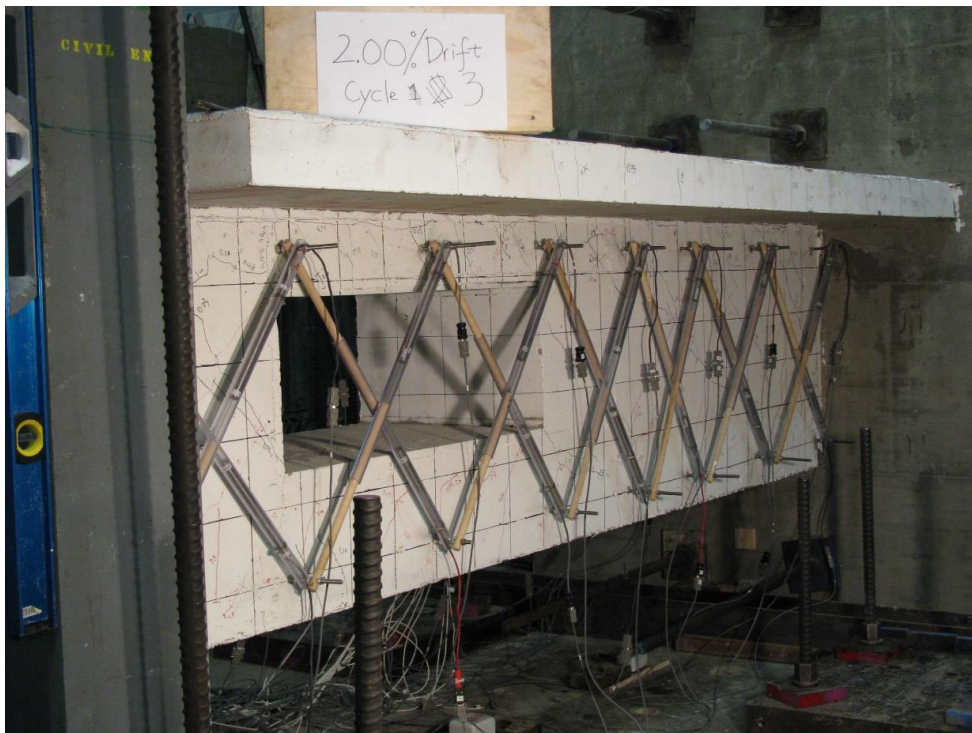
Figure 5.9: Crack pattern at 2.0% drift for S2
