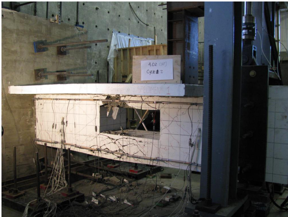
Figure 5.3: Crack pattern at 3.0% drift for S1
