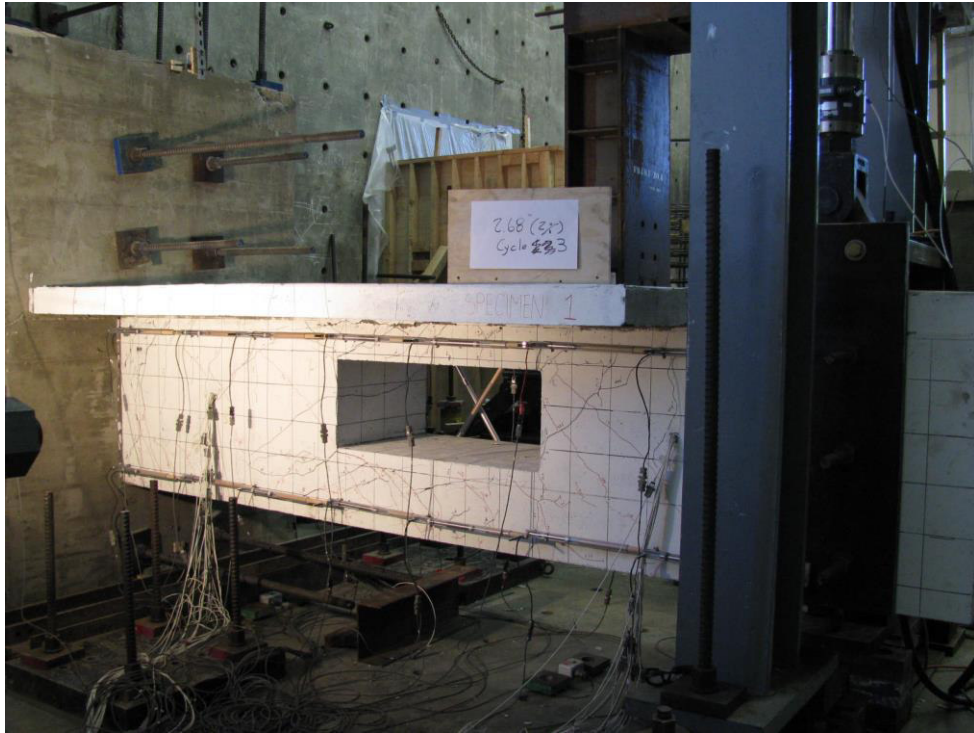
Figure 5.2: Crack pattern at 2.0% drift for S1
