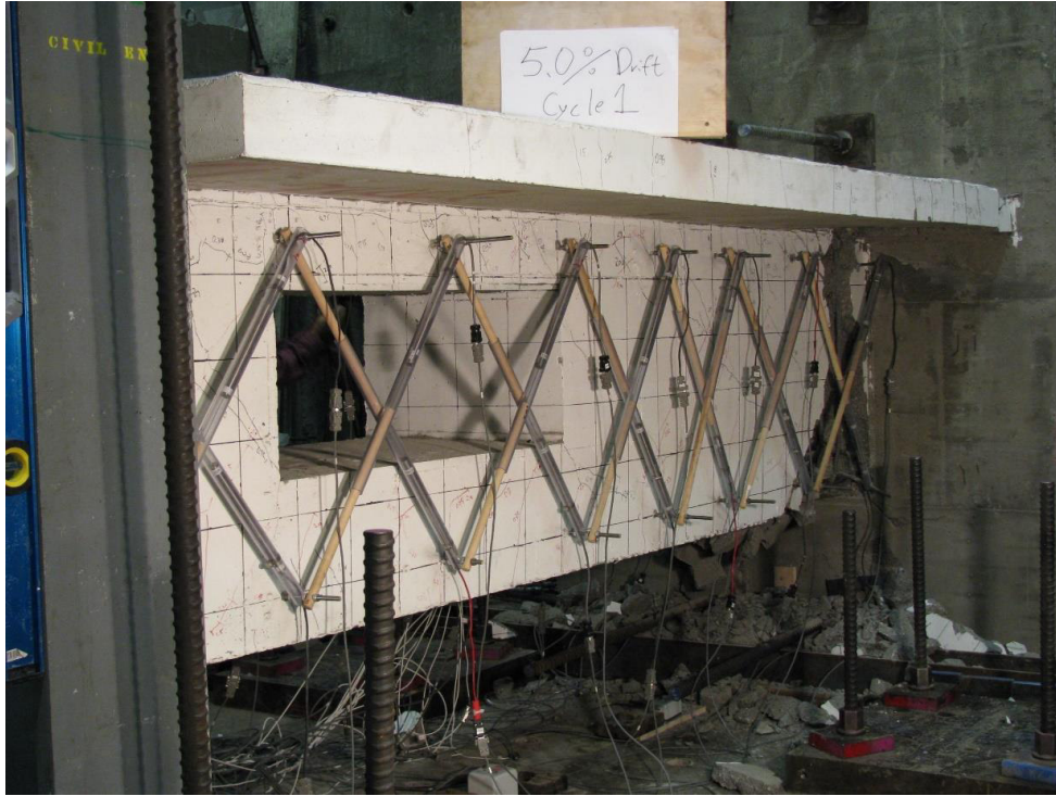
Figure 5.12: Crack pattern at 5.0% drift for S2
