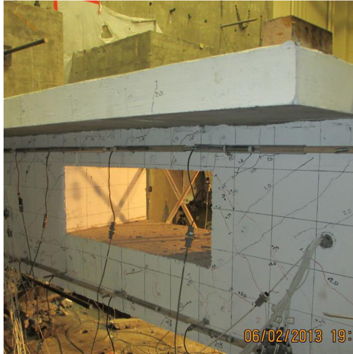
Figure 5.16: Opening region of S2 at end of test
