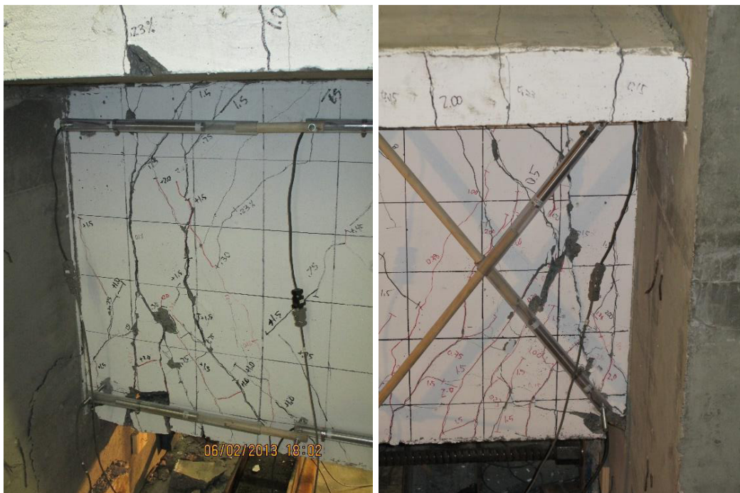
Figure 5.13: Cracking pattern at the fixed end at 2.0% drift on both sides of beam
