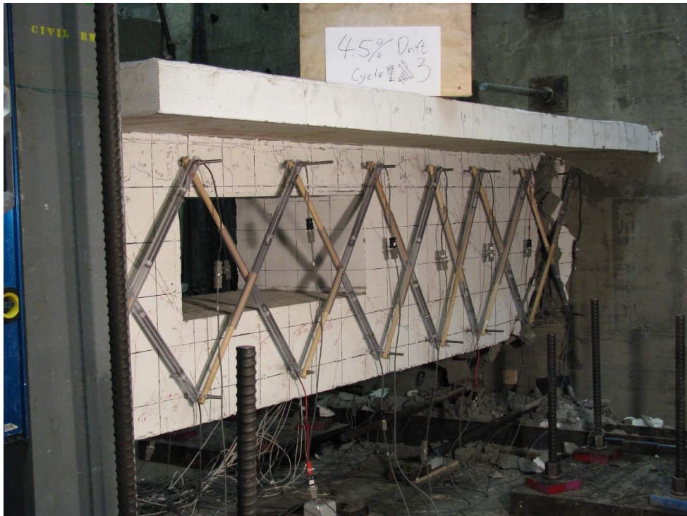
Figure 5.11: Crack pattern at 4.5% drift for S2
