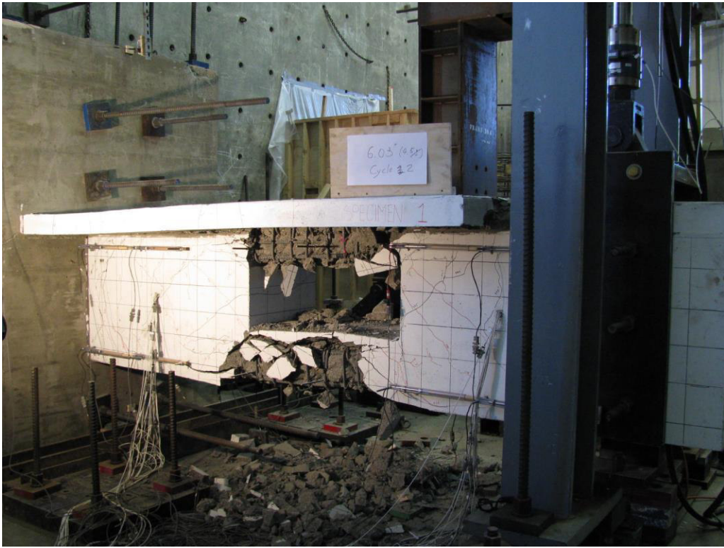
Figure 5.4: Crack pattern at 4.5% drift for S1
