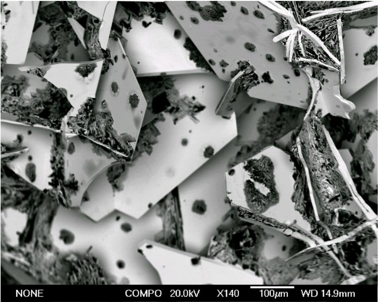
Figure 6.6: Backscattered electron SEM image of a fractured ingot of an arc-melted sample in the ratio W:B of 1:12. Light regions are the tungsten-containing phase.
