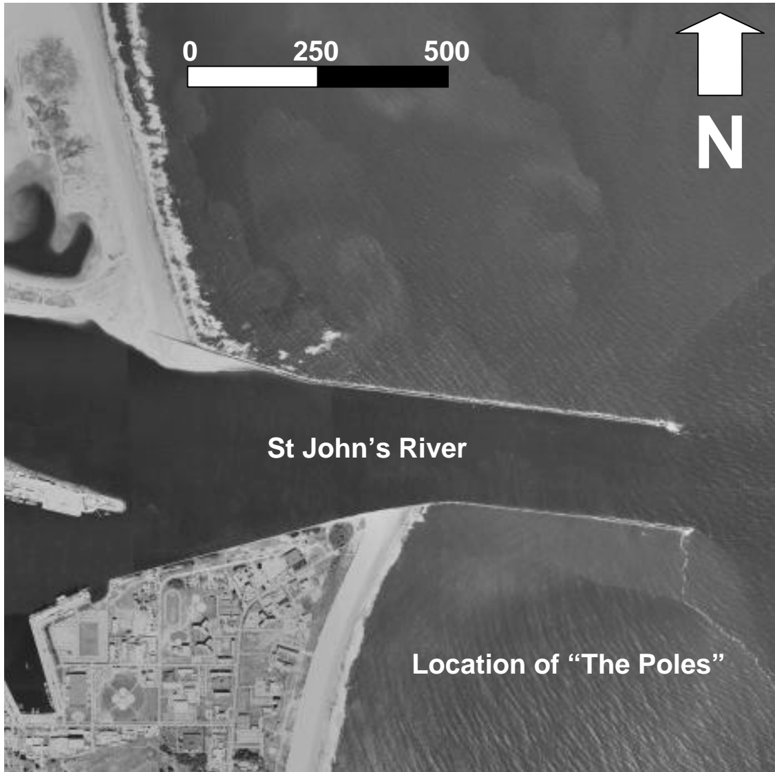
Figure 5-13. Aerial image of the jetties at the help create "The Poles" surfing break (Raichle, 1998).
