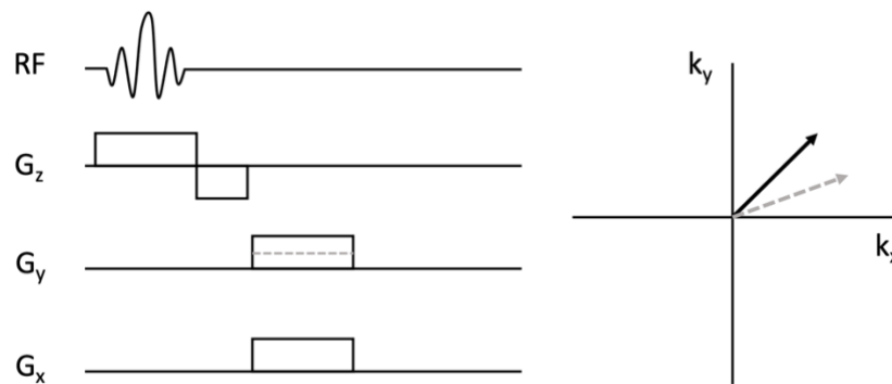
Figure 2.4. Sequence diagram of selective excitation with radiofrequency (RF) excitation, G_z slice selection, and readout of lines in k-space with G_y and G_x .
