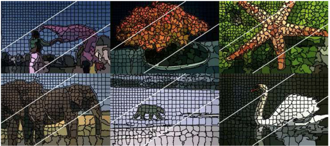
Fig. 2: Visual examples from the BSDS500 dataset. Each image is overlaid by three segments corresponding to 1000/500/200 superpixels using the proposed superpixel embeddings.
