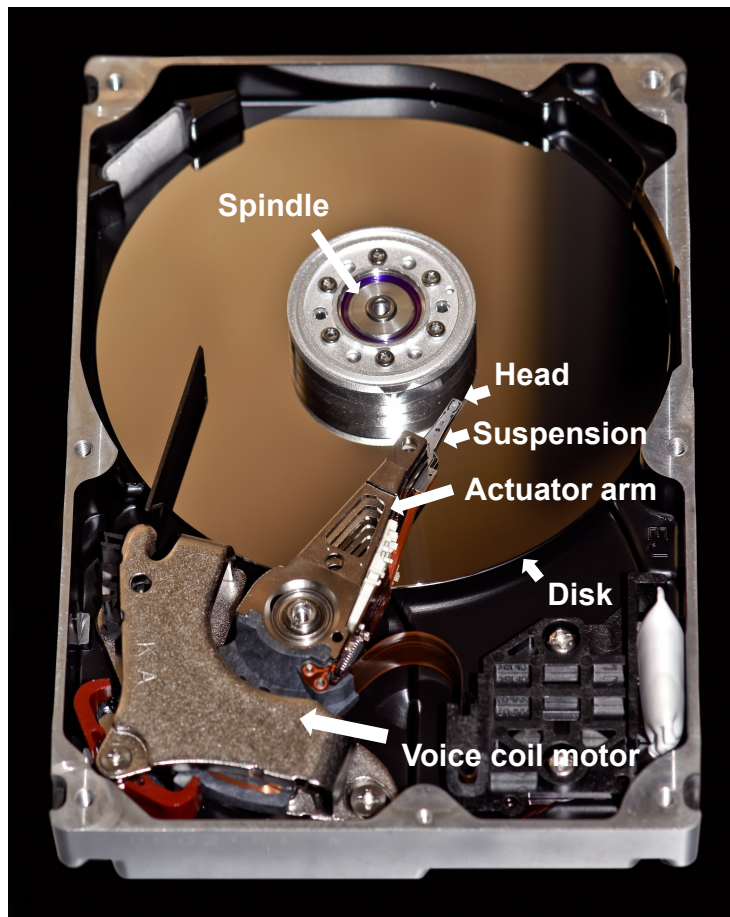
Figure 1.1: Internal view of a hard disk drive (HDD).
