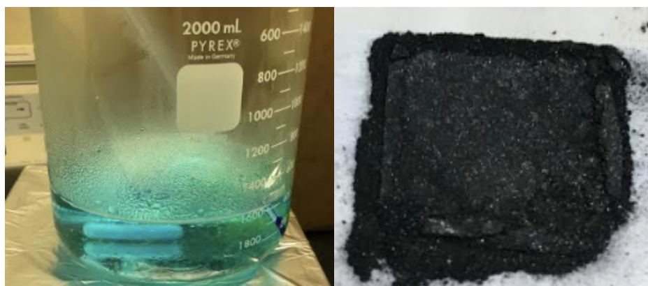
Figure 2.1: “Sol” step of CMAT synthesis stirred on a hot plate. Final annealed product mechanically pressed into a fine powder (less than 2 micron particles).
