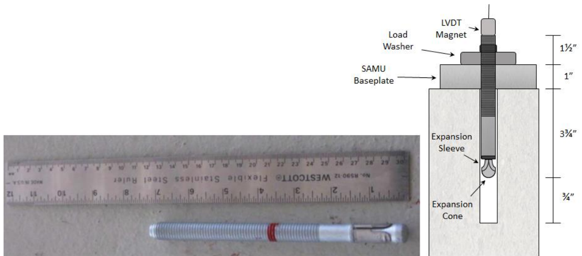
Figure 2-7: "N5" Expansion Anchor Pre-installation Picture and Installation Schematic
