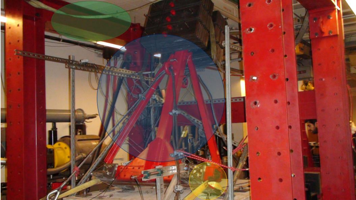
Figure 2-14: WALLE Catcher Systems for (a) Primary (blue), (b) Secondary (green), and (c) Tertiary (yellow)
