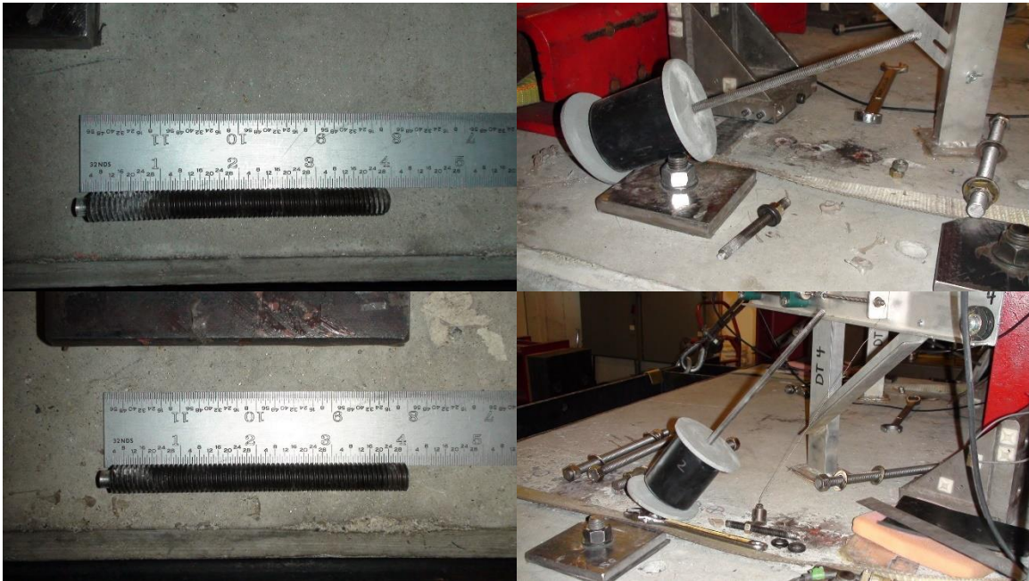
Figure 4-14: N3 Failure Photographs for A3 Anchor (top left) and Concrete Surface (top right) and A4 Anchor (bottom left) and Concrete Surface (bottom right) for BBM Test Sequence
