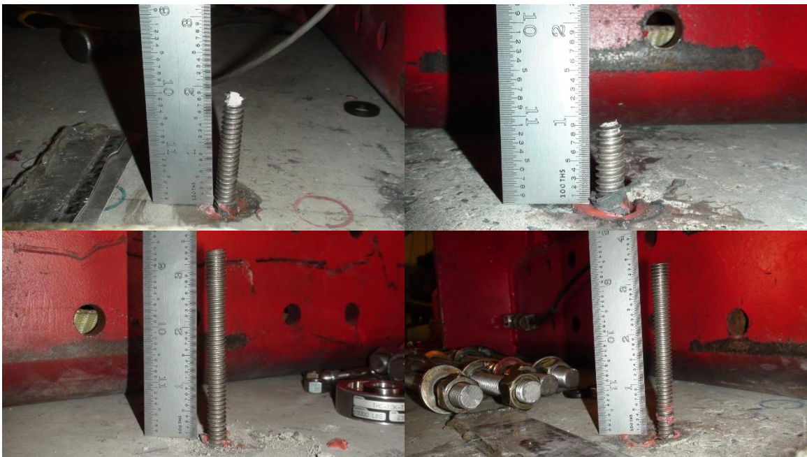
Figure 4-6: N1 Failure Photographs for A1 (top left), A2 (top right), A3 (bottom left), and A4 (bottom right) for BBM Test Sequence
