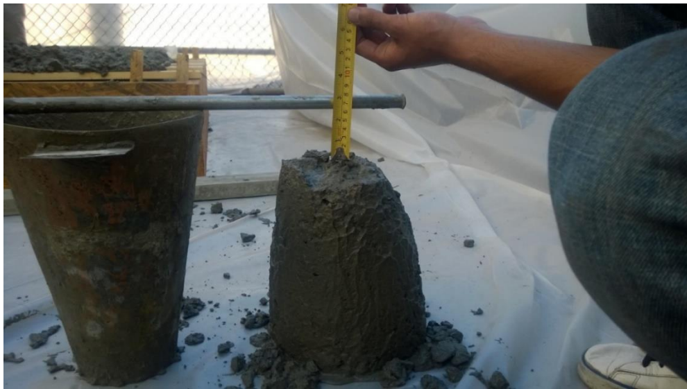
Figure 2-13: Slump Test Results for Concrete Slabs
