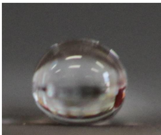
Figure 2.9 The profile for a water droplet on 10 nm Au composite structures
