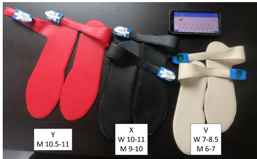
Figure 1: The Loadsol force sensing insoles used in the study and insole force data recorded via the Loadsol app on an Android device. Insole sizes are marked with manufacturer labeled sizes and corresponding US women's (W) and men's (M) shoe sizes.
