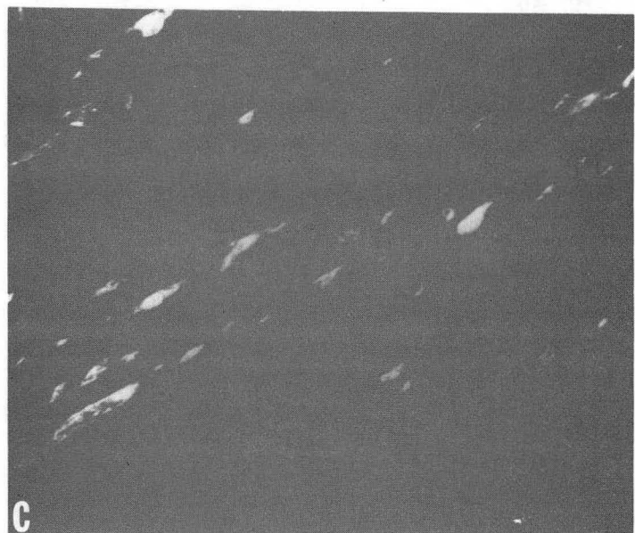
11. Transmission electron micrograph of 9Ni steel in the QT condition after 3% strain: (a) bright field; (b) dark field micrograph of martensite from mechanically transformed austenite; (c) dark field micrograph of remaining austenite. The variant of the fresh martensite differs from that of the surrounding packet.
