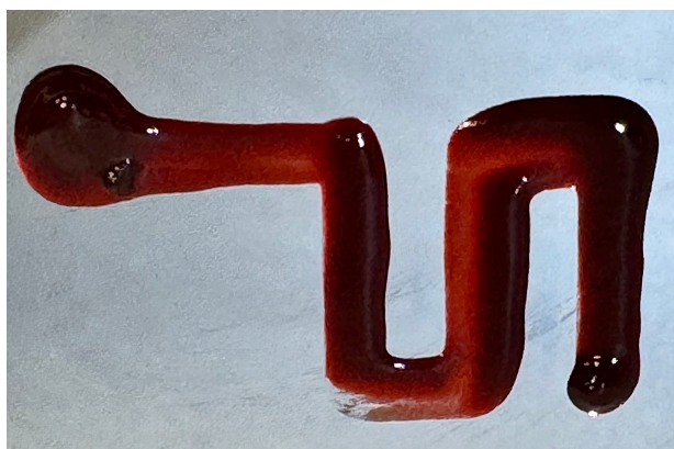
Figure 4.8. Photograph of a 3D-printed conjugated polyelectrolyte complex structure fabricated by direct-ink-write extrusion of the 80 °C CPEC fluid onto a silicon wafer. The printed serpentine pattern demonstrates robust shape retention and self-supporting line definition, confirming the suitability of the CPEC gel rheology for additive manufacturing of photoactive soft materials.
