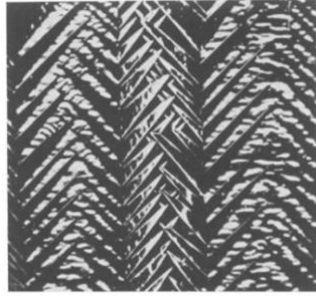
Figure 1.4 Photograph of magnetic domain structure in FeSi single crystal [5]
