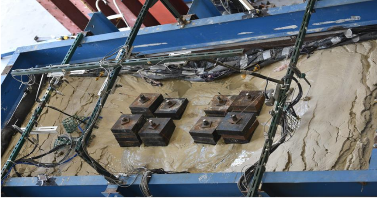
Figure 2.11. Observed soil-foundation system response prior to improvement
