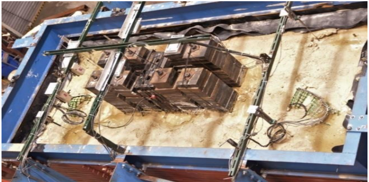
Figure 2.12. Observed soil-foundation system response after injection
