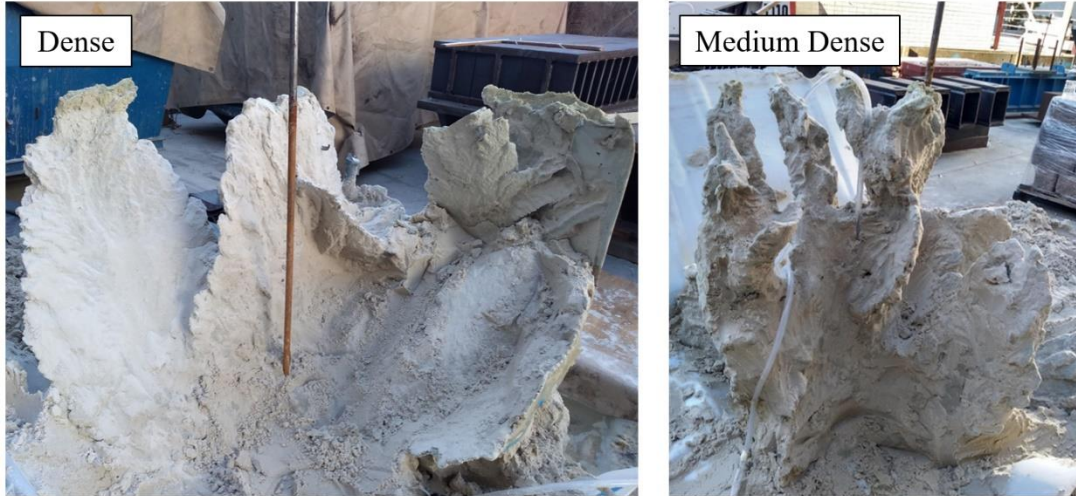
Figure 2.7. Observed composite inclusions (veins) after excavation in the dense and medium-dense specimens
