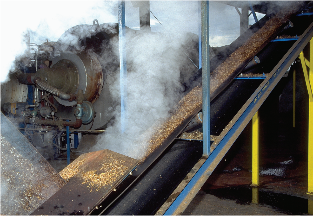
Figure 27. Wild rice exits the steam parboiler.
