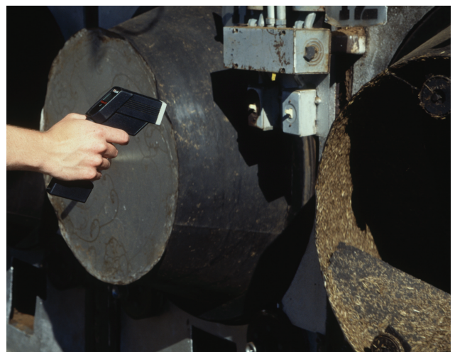
Figure 26. Using an infrared gun to monitor parching temperatures.
