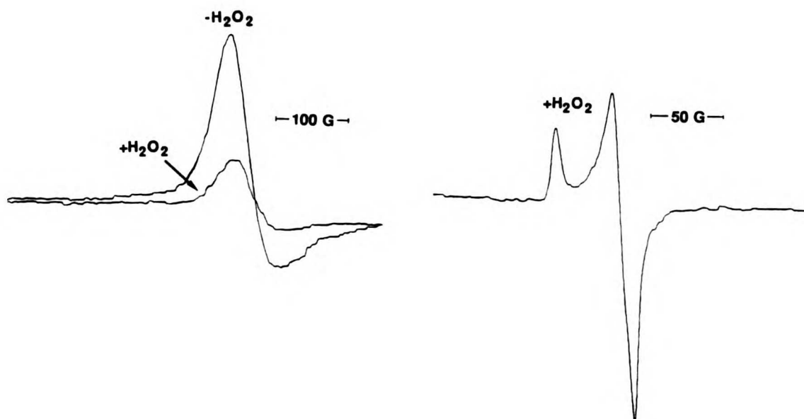
Fig. 2.11 The EPR spectra of horse myoglobin before and after addition of hydrogen peroxide (left trace, g = 6 region; right trace, g = 2 region).
