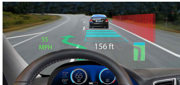
Figure 5: Augmented reality overlays information (often data) onto the environment as shown in this “heads up display”.
