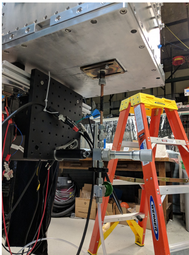
Figure 3.4: The water fill line, sealed by an ultratorr fitting and heated by nichrome wire. A shut off valve and Swagelok SS-4BMW vernier flow valve are used to regulate the flow of water into the buffer gas cell.
