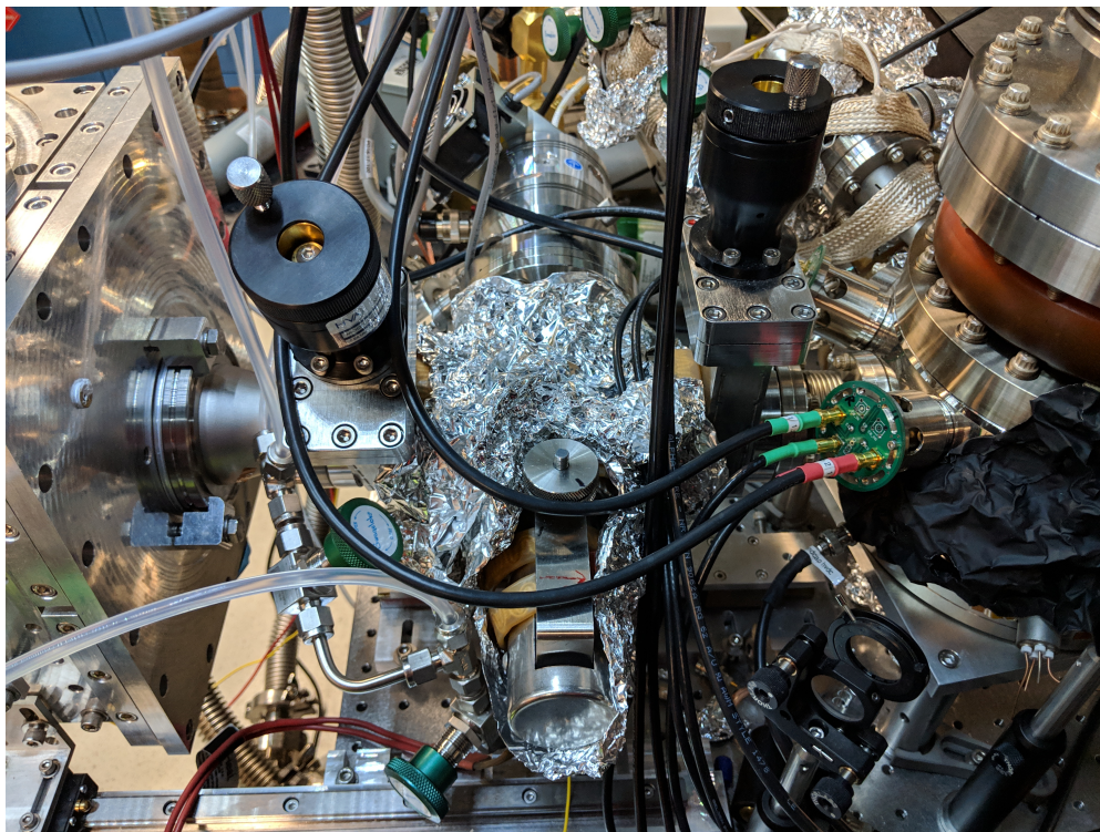
Figure 4.3: Differential pumping region in between the stem and ion trap chambers with gate valves on either end. Blank copper CF gaskets with apertures of 4 mm and 10 mm are placed towards the stem and ion chamber respectively to limit conductance of background gasses while allowing the cryogenic beam through. An Agilent Twistorr 84 FS turbo pump keeps the region at pressures around 10^{-10} Torr and a leak valve allows for controlled introduction of secondary gasses.
