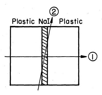
Fig. 6. Different -dE/dx for protons and electrons incident on NaI(T1) anticrystals in different directions (1) and (2).
