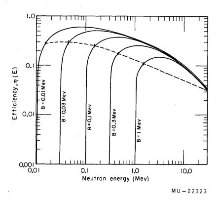
Fig. 1. Efficiency vs energy of plastic scintillator for d = 1 inch, and various values of B, plotted from Eq. (4) using a plastic density of 1.06 g/cm<sup>2</sup>. Dotted line above ( $E_{min}$  = 1.5 B) shows the useful neutron energy range for values of biased-energy B setting.
