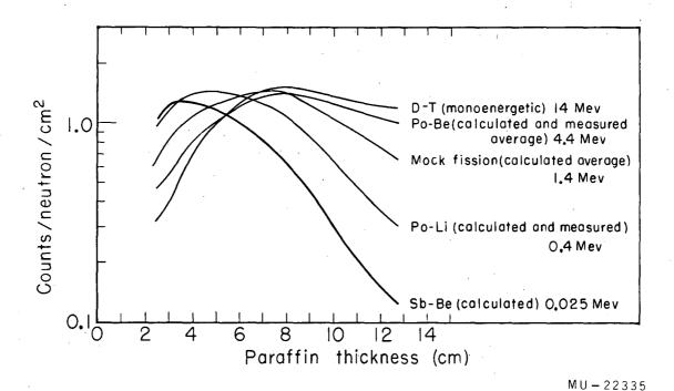
Fig. 9. BF<sub>3</sub> counting rate as a function of paraffin thickness for various neutron sources, corrected to an isotopic flux distribution. Entire assembly was covered with Cd (after Wallace et al see Ref. 29).
