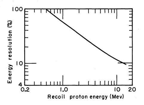
Fig. 2. Energy resolution vs proton energy, plotted from Eq. (6), using the nonlinear response of stilbene tabulated by Swaltz and Owen for KB = 0.012 mg/cm<sup>2</sup> in Birk's semitheoretical formula.
