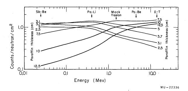
Fig. 10. Average efficiency of a BF3 proportional counter as a function of neutron energy for various paraffin thickness, corrected to an isotopic flux distribution. Assemblies covered with Cd averaging over the  $4\pi$  solid angle, have introduced error of up to 10% (after Wallace et al: see Ref. 29).
