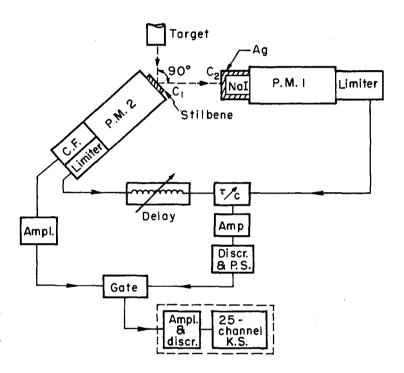
Fig. 7. Block diagram of spectrometer used by Beghian et al. employing two crystals with an Ag detector to select the direction of incident neutrons (see Ref. 22).
