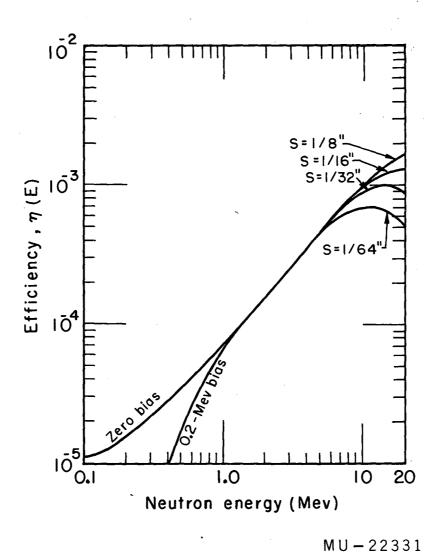
Fig. 11. Efficiency vs energy of a paraffin-moderated proportional counter for various paraffin wall thicknesses (after Moyer: see Rev. 30).
