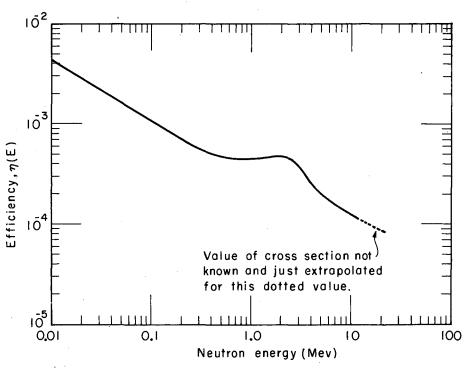
Fig. 8. Efficiency vs energy of He<sup>3</sup>(n.p)T proportional counter, plotted from Eq. (10) for d = 5 cm and 5 atmospheres of He<sup>3</sup>. Actual efficiency is smaller than plotted reaction probability.
