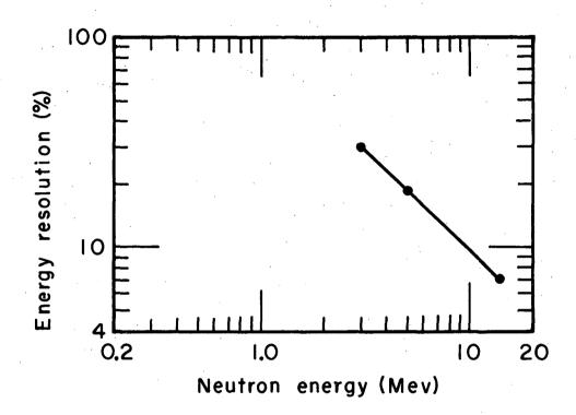
Fig. 5. Energy resolution vs energy of Li<sup>6</sup>I(Eu) scintillator.
