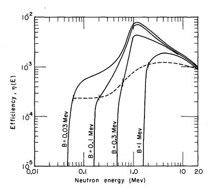
Fig. 3. Efficiency vs energy of He<sup>4</sup> scintillator counter, plotted from Eq. (7) for d = 10 cm and 5 atmospheres, for various values of B. The dotted line shows E<sub>min</sub> = 2B.
