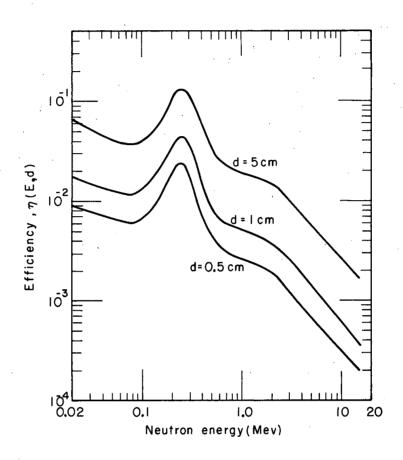
Fig. 4. Efficiency vs energy of Li<sup>6</sup>I(Eu) scintillator, plotted from Eq. (9) for various values of d.
