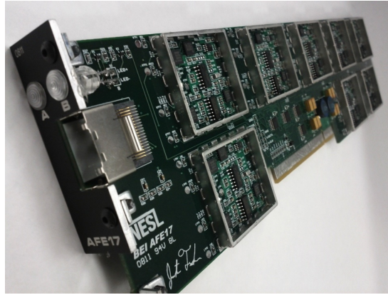
Figure 4.4: Each of the analog front end card contains 16 channels. Each channel has a programmable gain instrumentation amplifier and a programmable band-pass filter[Fri12]..
