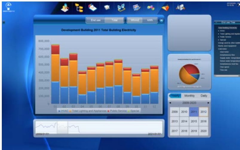
Figure 5.2 iSagy Total Building Electricity Use by Subsystem
