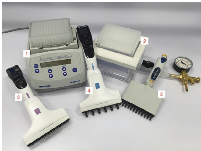
Fig. 1 Entry level high throughput liquid handling and processing equipment. (1) Small orbit (1.5–3 mm) high speed ( \sim 1000 rpm) shaker with 96-deep well block. (2) Vacuum manifold for 96-well filter plates. (3) Integra Viaflo variable span (4.5–9 mm) 12-channel pipettor. (4) Electronic fixed channel pipettor. (5) Manual fixed channel pipettor
