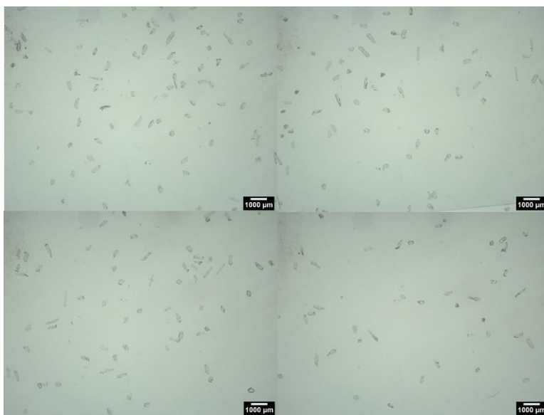
Figure S2. Optical microscope images of the 180 \mu\text{m} nominal crystals.
