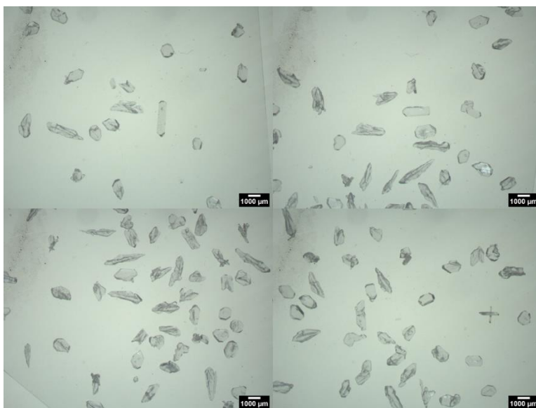
Figure S4. Optical microscope images of the 710 \mu\text{m} nominal crystals.
