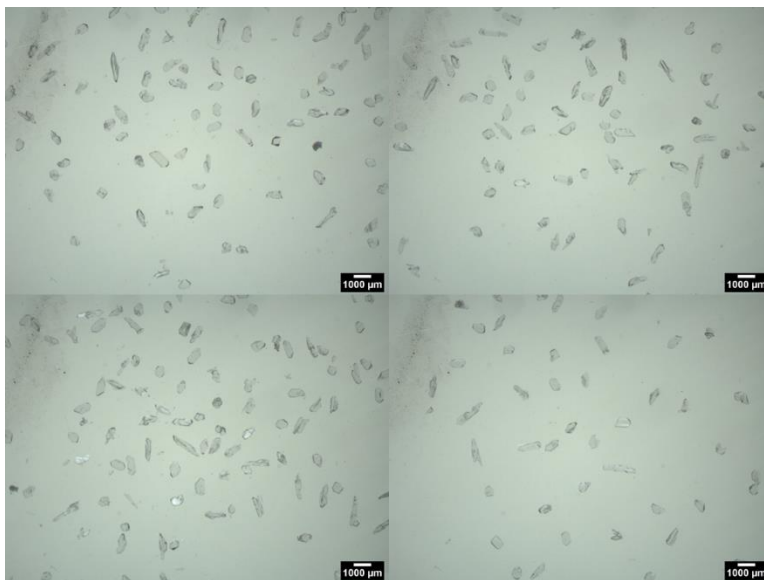
Figure S3. Optical microscope images of the 355 \mu\text{m} nominal crystals.
