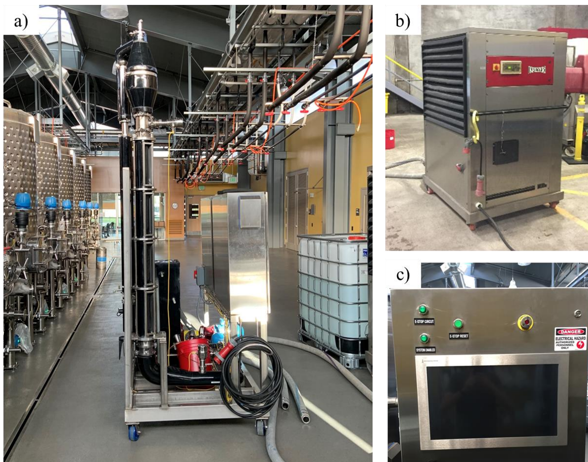
Figure 19. Photos of the completed fluidized bed system. a) The pilot-scale fluidized bed unit at the UC Davis research winery. b) Chiller used to chill incoming wine. c) Touch screen control panel.
