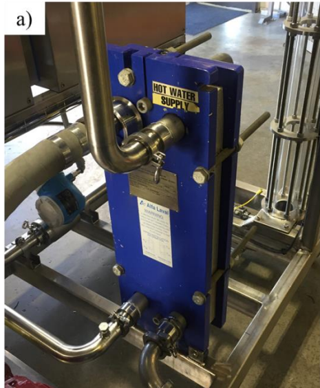
Figure S7. Photo of the plate heat exchanger for energy recovery. a) Heat exchanger on the unit before insulation was added. b) manufacture's information plate.
