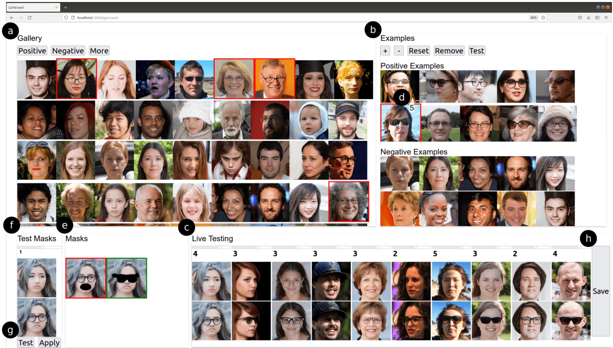
Figure 3.1: GANRAVEL enables users to disentangle editing directions in generative adversarial networks (GAN) using global and local disentanglement approaches. (a) A direction is often entangled when created by selecting exemplary images from the gallery. (b) The weights of the exemplary images can be adjusted to disentangle global attributes such as age and gender. (c) The direction can be tested on the live-testing section using multiple test images. (d) The user can hover over an exemplary image to see its weight and go back and forth between weight adjustments and live-testing until global attributes are disentangled. (e) The user can use masks to disentangle local attributes such as glasses and closed mouth. (f) The masks can be combined to either preserve or discard a region of interest and they can be tested. (g) Resulting disentangled direction can be applied to other test images in the live-testing section. (h) The final disentangled direction can be saved and applied in other future images.
