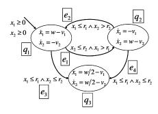
**Fig. 4.** A more complete hybrid system model of the water tank system.
