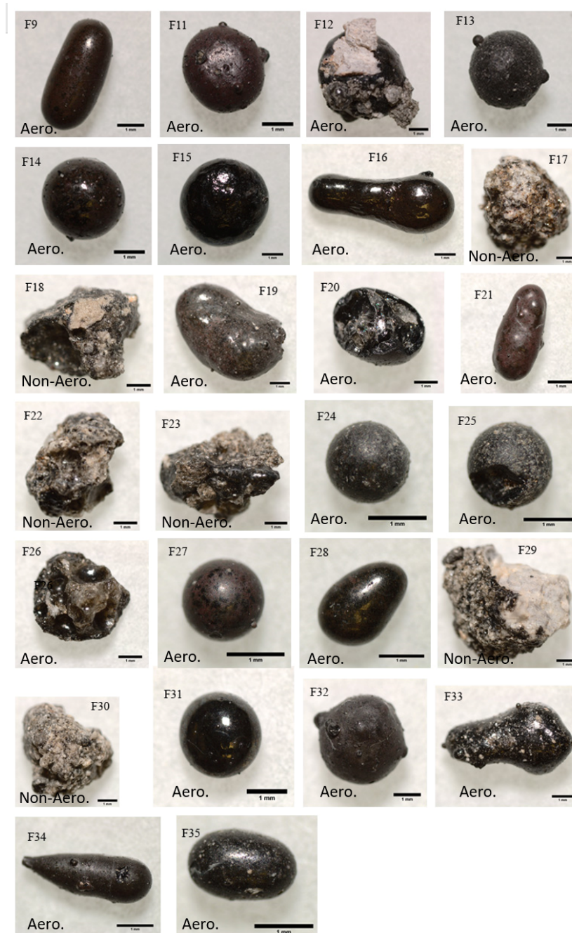
Figure 3.1: Optical images of all fallout samples used in this study. Samples with smooth continuous surfaces are labeled 'Aero.' for aerodynamic, and samples with irregular surfaces are labeled 'Non-Aero.' for non-aerodynamic.
