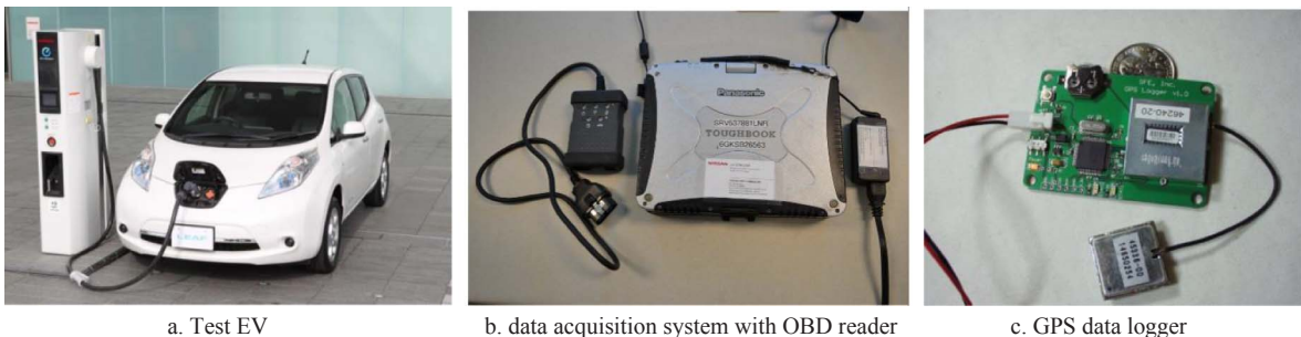
Fig. 4. Test Vehicle and Data Acquisition Equipment.
