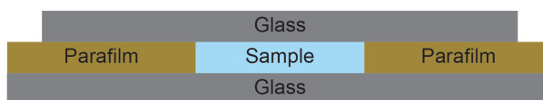
Figure A.4: Typical flow cell. Flow cells were utilized as simple sample holders that allowed microscopic visualization.
