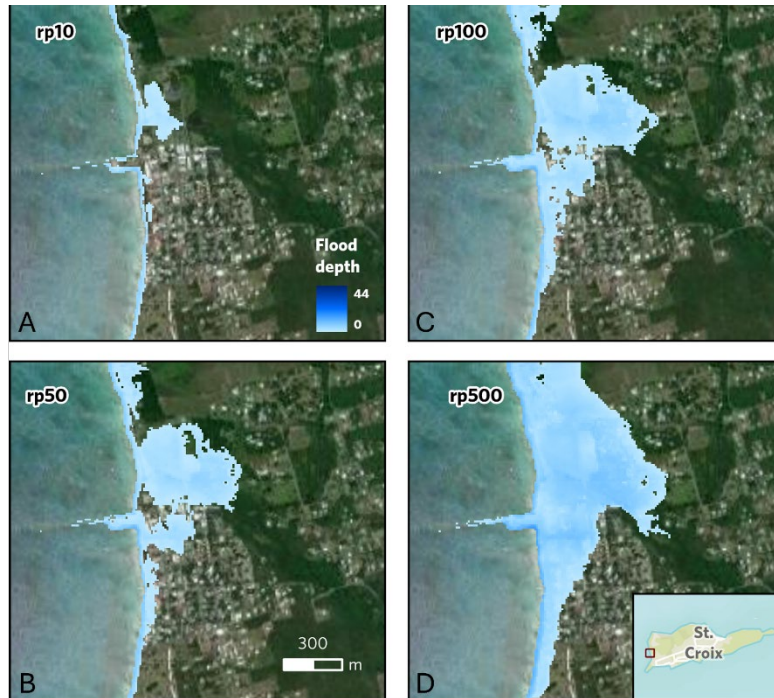
Figure 7. Maps showing example 10-meter resolution flood depths for various storm recurrence intervals on St. Croix, U.S. Virgin Islands. A , 10-year storm. B , 50-year storm. C , 100-year storm. D , 500-year storm. Colors indicate flood-water depth, in meters, interpolated from adjacent XBeach model profile model transects spaced every 100 meters along the coast. Satellite image extracted from Esri, Maxar, Earthstar Geographics, and the GIS User Community.
