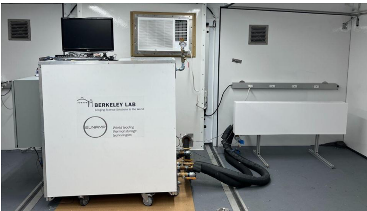
Figure 1: Indoor view of the structure (left) with thermal energy storage and controls systems and fan coil unit; and outdoor view (right) with HP unit. Note the default PTAC unit (through wall) that the experimental HP TES replaces.
