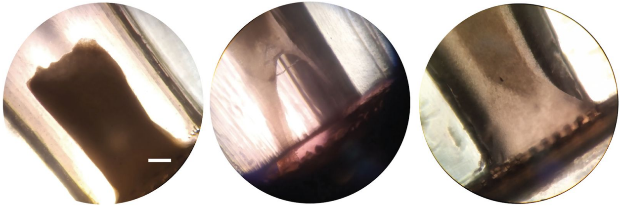
Figure 5. Myobundle comparisons. Images from left to right: Complete detachment from one end, partial tearing at one end, successful concave shape at binding point. (Scale Bar 1mm).
