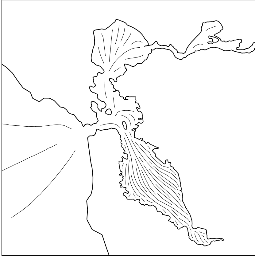
Figure 3.13: Flow-aligned contours, traced from the principal velocities, ready for input to the re-gridding process. The separation between adjacent contours scales with the grid resolution, leading to sparser contours in the north and west.
