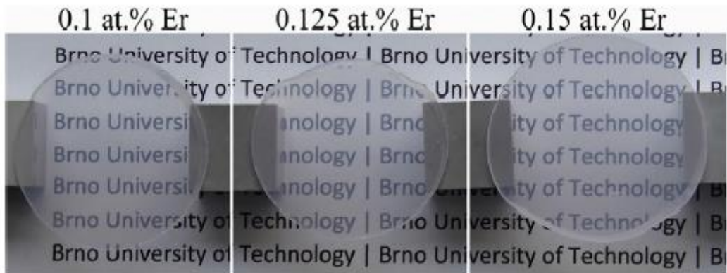
Figure 2.5. Transparent Er 3+ doped alumina fabricated through the HIP-ing method [28].
