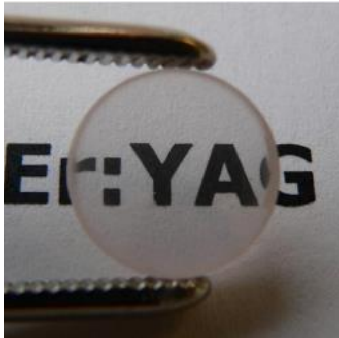
Figure 2.3. Optical picture of the polished Er:YAG ceramic sample demonstrating the high transparency capable with this material system [35].
