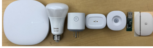
Figure 4.9: Smart devices and ZigBee packet sniffer used in our testbed for evaluating IOTGAZE.
