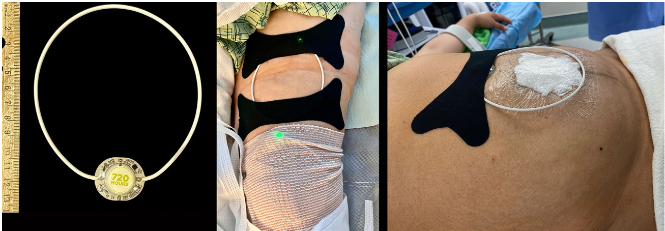
FIGURE 1 A wearable pulsed shortwave therapy device with a pulse generator and flexible 12cm-diameter antenna. The unit is secured with an included cotton-based kinesiology or paper tape. The single control is an on/off button on the back of the pulse generator, and the green light emitting diode indicates the unit is activated. Imaged are knee arthroplasty and umbilical hernia repair. Used with permission from the first author.
