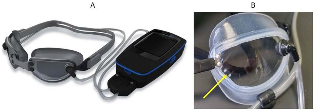
Figure 1. Overall design of the multi-pressure dial (MPD) system used in this study. As demonstrated in “A”, each side of the goggle makes a separate seal around the periocular space and can be adjusted to a specific target pressure that is independent from the contralateral side. “B” shows the location of small holes (yellow arrow) drilled in the medial sides of the goggle that enables clear anterior surface of the lens during the imaging procedure.
