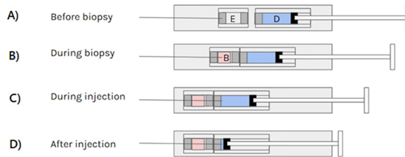
Fig 1. Principal and operation of VitreoDx device. In its initial state A), the double ended needle fixed into the outer housing has an interior septum piercing end which is buried in the distal septum of the evacuated sample container 'E'. A drug cartridge 'D' with a distal septum and a plunger sits proximally adjacent to the sample chamber. Depressing the plunger to a first stop transitions the device to an aspiration state B) by advancing the cartridge and the sample chamber such that the needle pierces the sample chamber and applies vacuum to needle, thereby aspirating a liquid biopsy 'B'. Further depressing the plunger moves the device into a injection state C), advancing the cartridge and the sample chamber until the needle pierces the drug cartridge. At this point, any further depression of the plunger acts to force any drug contained in the cartridge out of the needle until the device reaches a completed state D). Note that drug cartridge was, for the experiment described here, empty to avoid introducing non-vitreous fluid to the eye.
