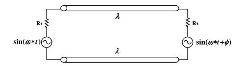
Figure III.19: Simulated waveform of two sources shunted by one wavelength long transmission line
