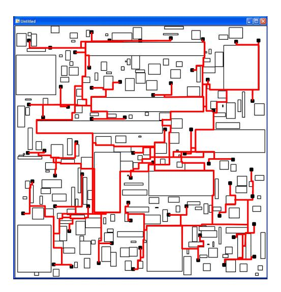
Figure III.15: Clock tree for a 200K flip-flops, 200 obstacles chip top level route are shown, small black squares indicate the root of local routing trees
