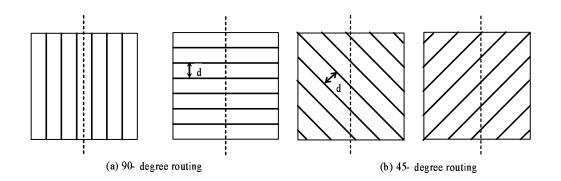
Figure II.8: Explanation of throughput increase for a 45-degree mesh
