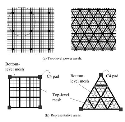
Figure II.13: Power distribution networks and representative areas for M- and Y-architectures.
