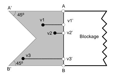
Figure III.11: Shadow region and direct virtual node insertion
