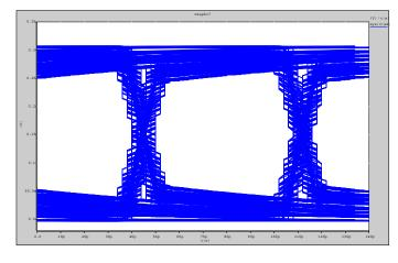
Figure IV.7: Eye diagram of the output voltage for a 4 stage 2cm-length surfliner
