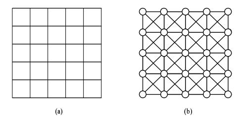
Figure II.3: A 90-degree and 45-degree mixed mesh of n = 5
