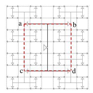
Figure III.2: An H-tree with A Two Level Mesh
