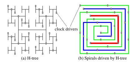
Figure III.17: Multi-level Tansmission Line Spirals Network
