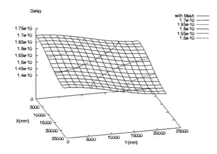
Figure III.8: Delay of leaf nodes on an H-tree with multilevel meshes
