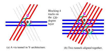
Figure II.16: Via tunnels and bank of via tunnels in Y-architecture.
