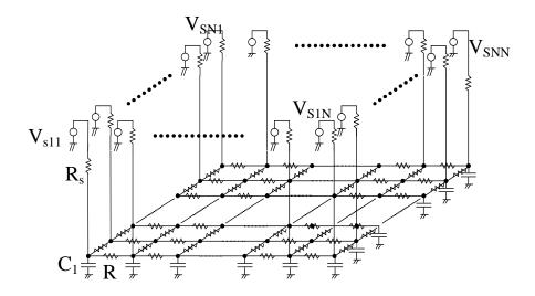
Figure III.6: Circuit model used to calculate the skew on a mesh
