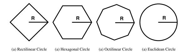
Figure A.1: Circles with radius R for each routing geometry (rectilinear, hexagonal, octilinear and Euclidean).
