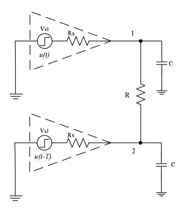
Figure III.3: simplified Circuit Model of RC Shunt
