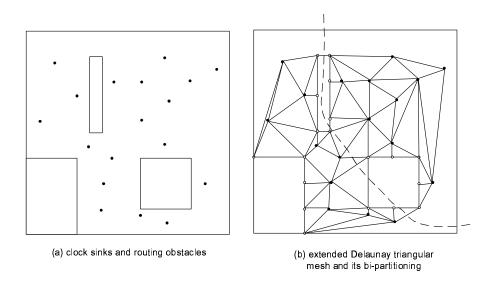
Figure III.13: Extended Delaunay Triangulization and a Bi-Partitioning of Triangular Graph
