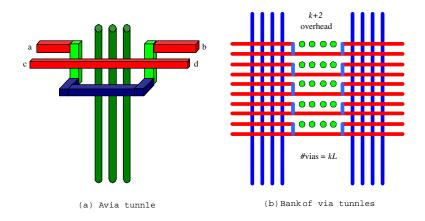
Figure II.15: Via tunnel and bank of via tunnels in the M-architecture.
