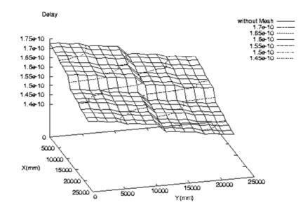
Figure III.7: Delay of leaf nodes on an H-tree without mesh
