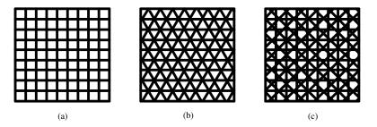
Figure II.14: Routing grids in M-, Y- and X-architectures.
