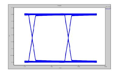
Figure IV.8: Eye diagram of the output voltage for a 120 stage 2cm-length surfliner
