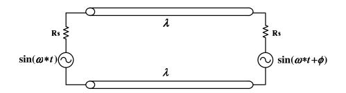
Figure III.18: Two sinusoidal sources with phase shift shunted by a wavelength long transmission line
