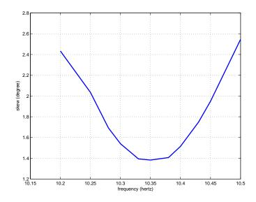
Figure III.24: Frequency response of the transmission line network: skew  $\sim$  frequency relation
