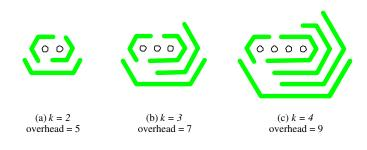
Figure II.17: Via tunnels with vias aligned in a line in Y-architecture.
