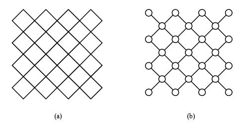
Figure II.2: Example of 45 degree mesh of n = 4
