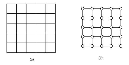
Figure II.1: A 5 by 5 communication mesh and its graph representation
