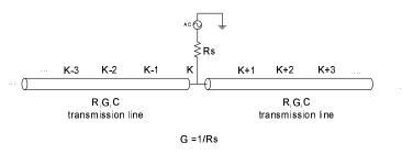
(b) continuous approximation of the circuit when only the k<sup>th</sup> driver takes effect
