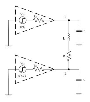
Figure III.16: Two clock drivers shunted by a lumped RLC line
