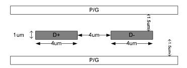
Figure IV.6: Implementation of Wires
