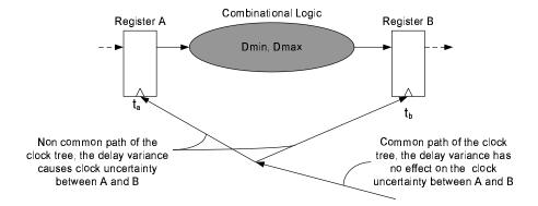
Figure III.9: Clock Uncertainties and Timing Constraints in Sequential Circuits
