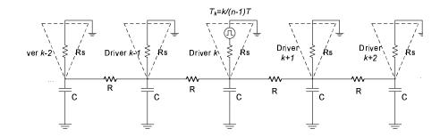
(a) Discrete RC circuit model when only the k<sup>th</sup> driver takes effect
