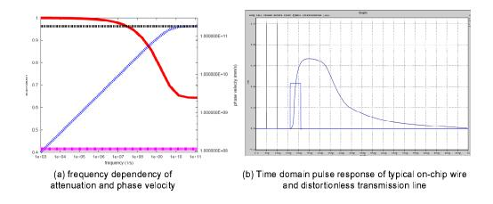
Figure IV.2: The attenuation and phase velocity v.s. frequency for a on-chip wire
