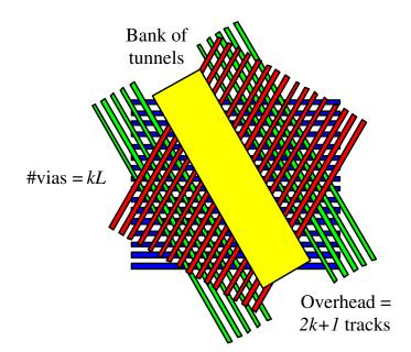
Figure II.19: Bank of via tunnels in Y-architecture.
