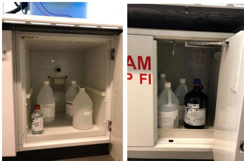
Figure 9. (left) Acid bottles with labels are stored in plastic corrosion-free cabinet, and organic ones are stored in steel cabinet.
