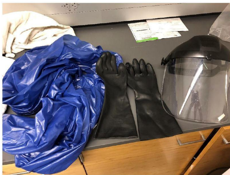
Figure 10. PPEs. (left to right) Blue chemical-proof coveralls, black nitrile gloves, and face mask.
