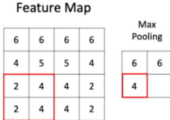
Figure 30: Max Pooling, 2D with 2x2 Filter
