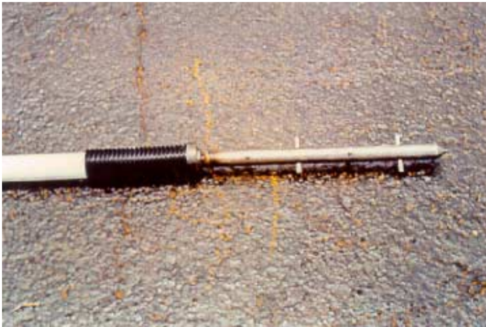
Figure 2.9. Anchor assembly of the MDD installation set in concrete at depth of about 3 meters (after CSIR).
