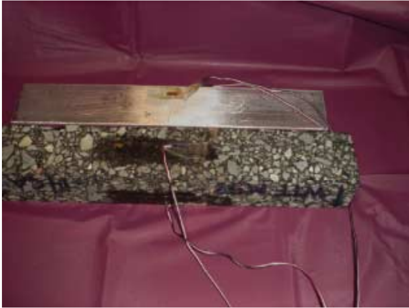
Figure 3.7. Strain gages attached on beam and aluminum support.
