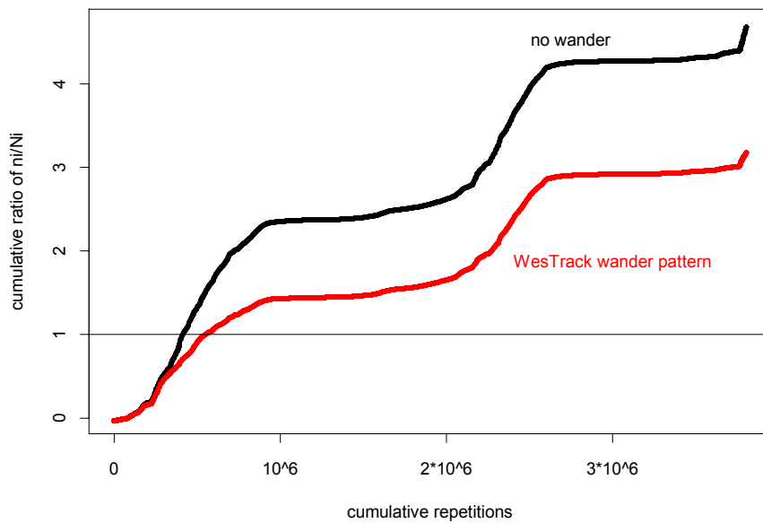
Figure B.6.19. Simulation result of crack initiation for WesTrack Section 11 (fine-plus, AV = 7.9 %, AC = 5.99 %).
