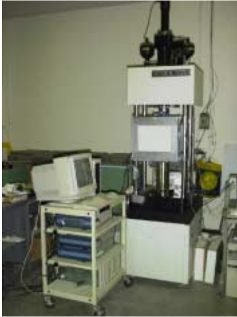
Figure 3.3. Modified fatigue test setup with temperature control box.
