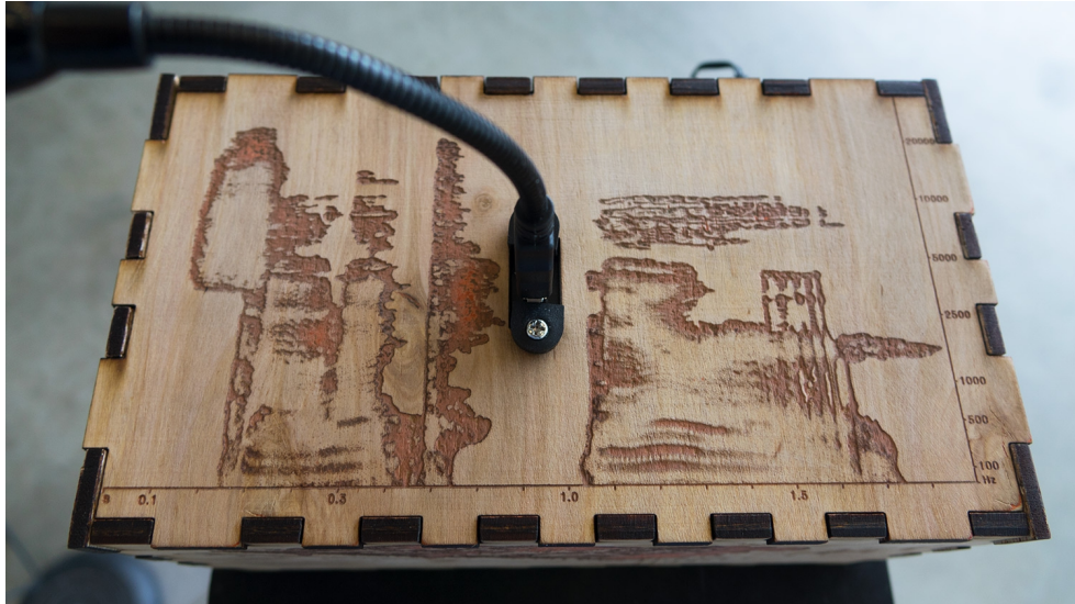
Figure 15: Laser engraving of 2D spectrogram on top face of wooden Sonic Mirror enclosure
