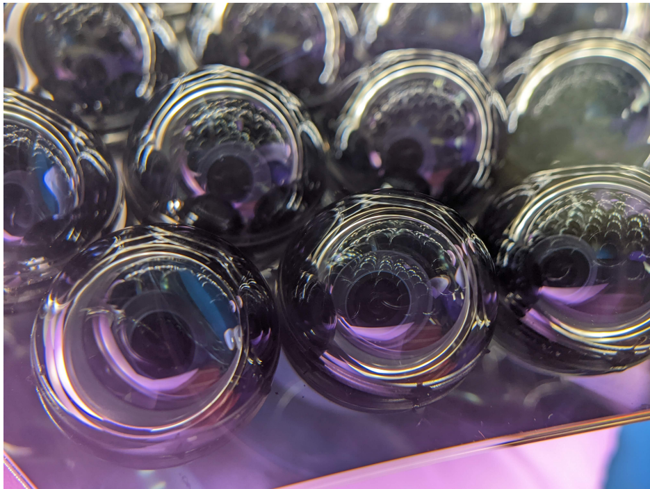
Figure 4.1: Close up of an SO-LF lenslet array. Here, silicon lenslets with a single-layer glass AR coating are used. The full array can be seen in the reflections on each lenslet.
