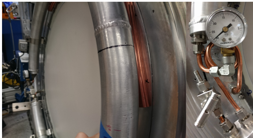
Figure 3.6: (Left) The volume expansion tube on the sky-side of the HWP and (right) the vacuum plumbing with the gauge used to monitor pressure.
