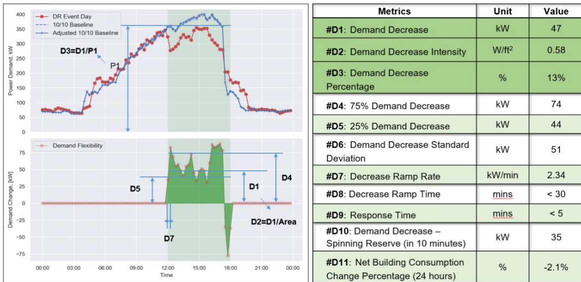
Figure 1. Proposed demand flexibility metrics for Load Shed with an example from an actual building DR event.
