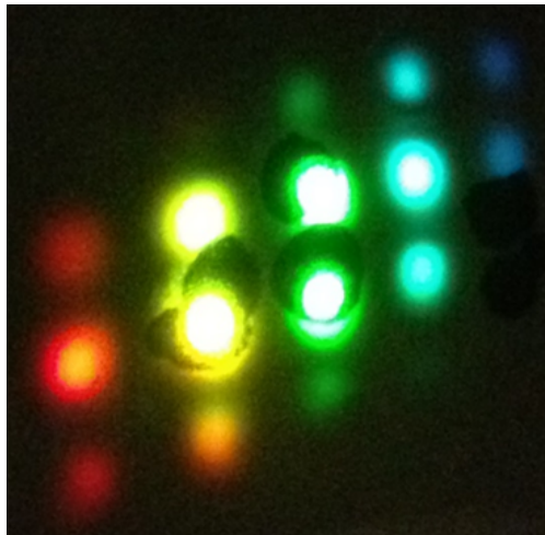
Figure 3.11: The diffraction pattern generated when all three NOPAs are mixed via BOXCAR geometry in space and time on a thin piece of glass. Presence of higher order diffractions depict the relative healthiness of the temporal and spatial profiles of each pulse. The more observed orders the better the spatial and temporal profiles of pulses. There are less diffractive orders than in the previous Figure because of the lower degree of overlap between the pulses due to different colors having a smaller coherence time as opposed to two degenerate colors.
