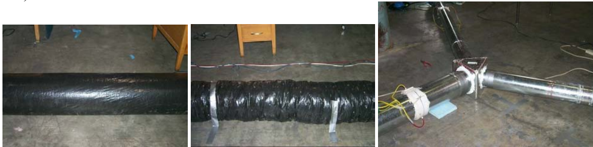
Figure 1. Stretched and compressed 10" (250 mm) flexible duct and splitter box test specimens.
