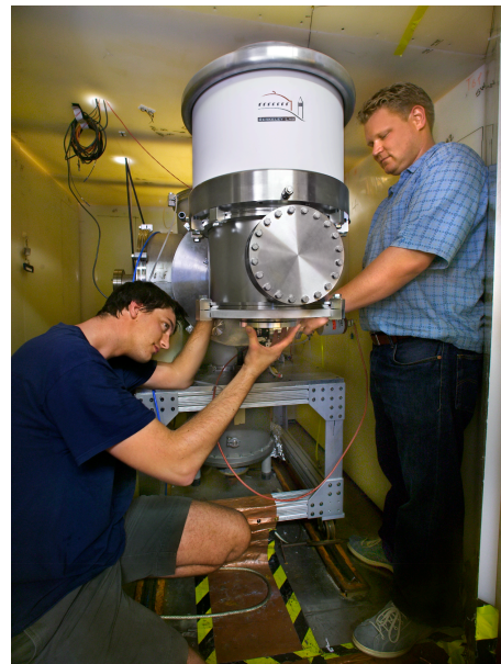
Figure 5-6: A CAD rendering (left) shows the main components of the co-axial neutron generator. On the right the neutron generator is shown being installed on a test stand.
