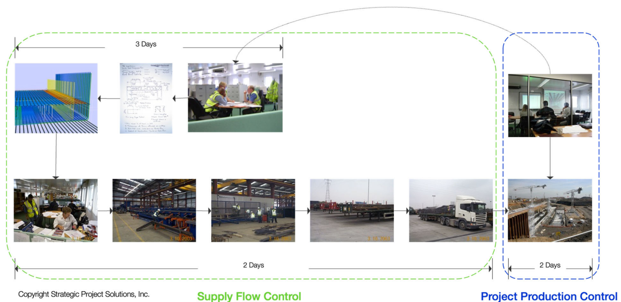
Figure 6: Rebar production system deployed to deliver Heathrow T5
